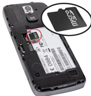
**Tip:** Take care not to scratch or bend the contacts on the memory or SIM card when inserting them into the card holders.
